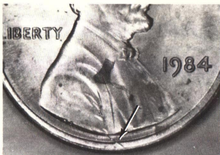
Figure 2: Die crack at the base of Lincoln's bust on a 1984 cent.
